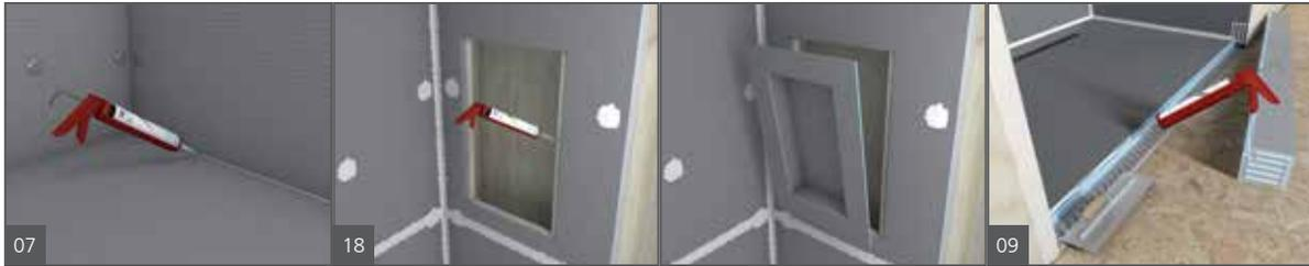
7. Apply continuous 1/2 in. (12.7 mm) beads of sealant between all connections of panels and install with tightly butted seams. Excess sealant must be spread flat with a putty knife. All seams and fastener heads in the assembly are covered with a secondary 1/2 in. (12.7 mm) bead of sealant and spread flat. The seams should be covered 1 in. (25.4 mm) on either side of the seam. All fastener/washers should be covered with sealant stretching 1 in. (25.4 mm) over the washer edges.
