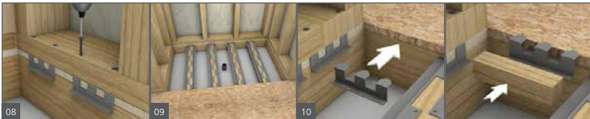
8. Make sure the C Brackets are mounted in a level position (assuming a level base plate), and use the longer Phillips self-drilling screws with wings provided by wedi. Fasten through the base plate and into the two metal claws resting between the base plate and the wood floor top.
