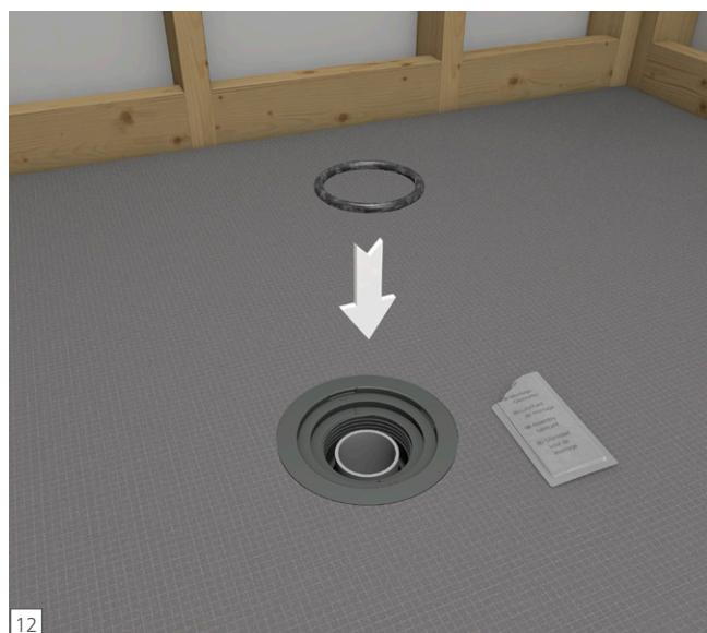
**EN** Apply wedi provided safe lubricant to the Rubber Sealing Gasket and insert the Rubber Sealing Gasket between the wedi Drain Unit's interior and the outside of the 2 in. waste pipe in the floor. Push the Rubber Sealing Gasket down along the waste pipe until it is stopped by the Drain Unit's lower interior flange.
