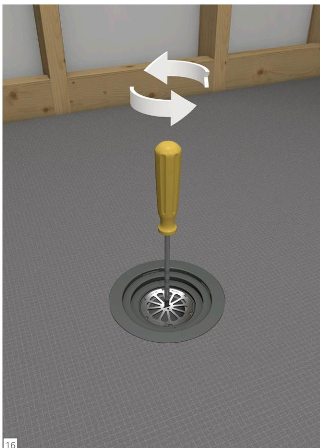
**EN** Insert a flat headed screwdriver into Strainer Key slit and turn **LEFT** to tighten the compression seal (turn Counter-Clockwise). Achieve a hand-tight fit and do not over-tighten.
