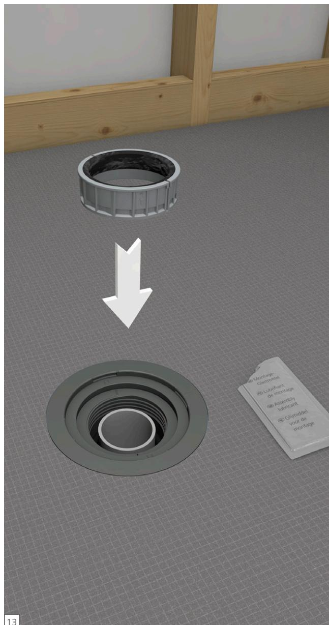
**EN** Apply wedi provided safe lubricant to the rubber part of the Compression Spacer. With the rubberized part pointing up now insert the Compression Spacer in between Drain Unit and waste pipe and on top of the Sealing Gasket. The Compression Spacer will push the Rubber Sealing Gasket down into its resting position. The Compression Spacer's rubberized part will not always sit flush with the floor waste pipe's edge, which is due to the thinset thickness tolerances under the shower base.
