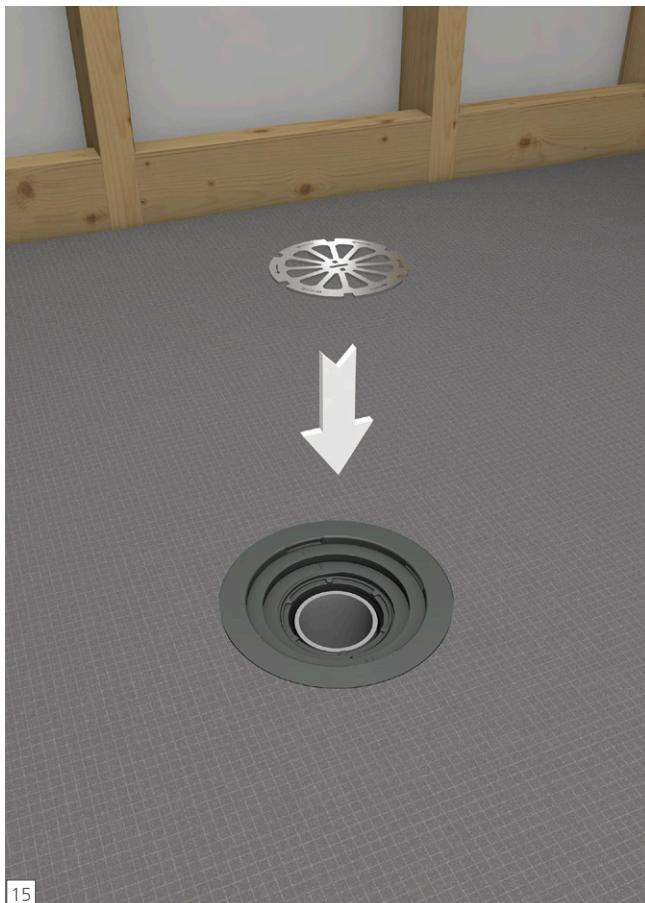
**EN** Insert Strainer Key into Locking Nut at notch connections and with Strainer Key printed side up. The Strainer Key is used as a tool to tighten the compression seal of the Drain Unit, but remains in place later to serve as a hair catcher to protect the drain and make maintenance and cleaning easy.
