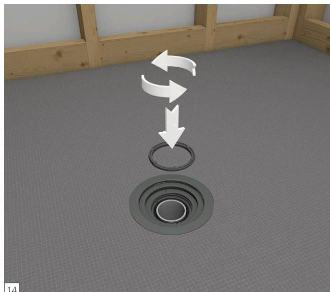
**EN** Insert the Locking Nut with notched side up into the threaded part of the Drain Unit opening and screw down until Locking Nut top is flush with top edge of Drain Unit's threaded part. **Important: Turn Locking Nut to LEFT to insert and screw into flush position (turn Counter-Clockwise).**
