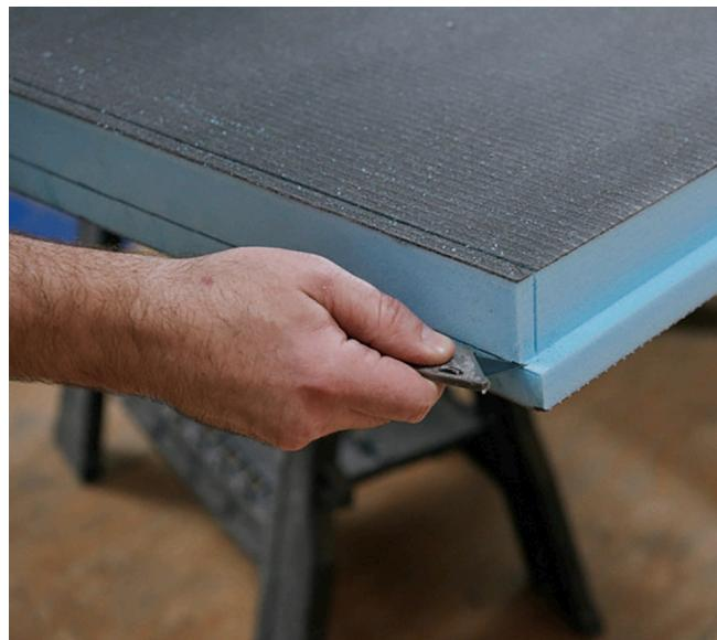
**EN** A wedi shower base can be cut to size using a circular saw with standard carbide blade. You can remake the 1/2 in. x 1/2 in. perimeter channel by cutting through the cement surface using the circular saw set to cut 1/2 in. deep. You can use a sharp utility knife to cut the new channel 1/2 in. wide through the blue exposed foam side. Clean the new channel and the base and remove all saw dust and loose particles.
