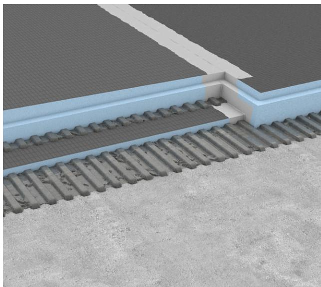
**EN** wedi shower bases thicker than 1 1/2 in, where an extension is connected require a wedi building panel be placed and thin-set mortar adhered under the extension panel to adjust for a proper connection fit.
